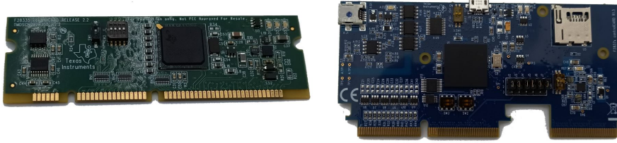
Figure 4: TMS320F28335 control card of the 1 kW converter (left) and TMS320F28379D control card of the 2 kW converter (right)
